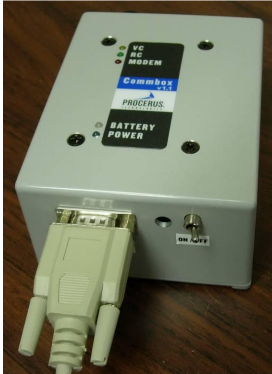
Figure 8. RS232 cable connected to Commbox.
